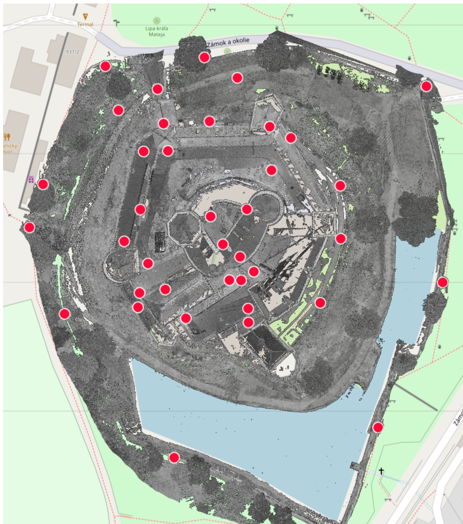
Figure 2. Scanning plan based on the digital map of the area.
