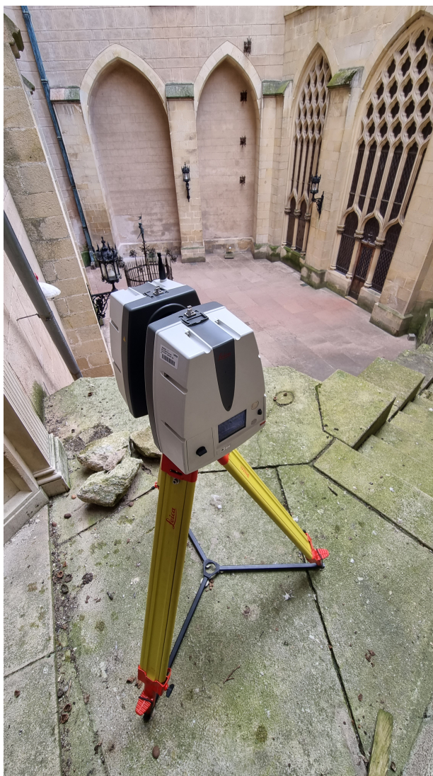
Figure 1. Laser scanner Leica P30 in field conditions during scanning of the Bojnice Castle.
