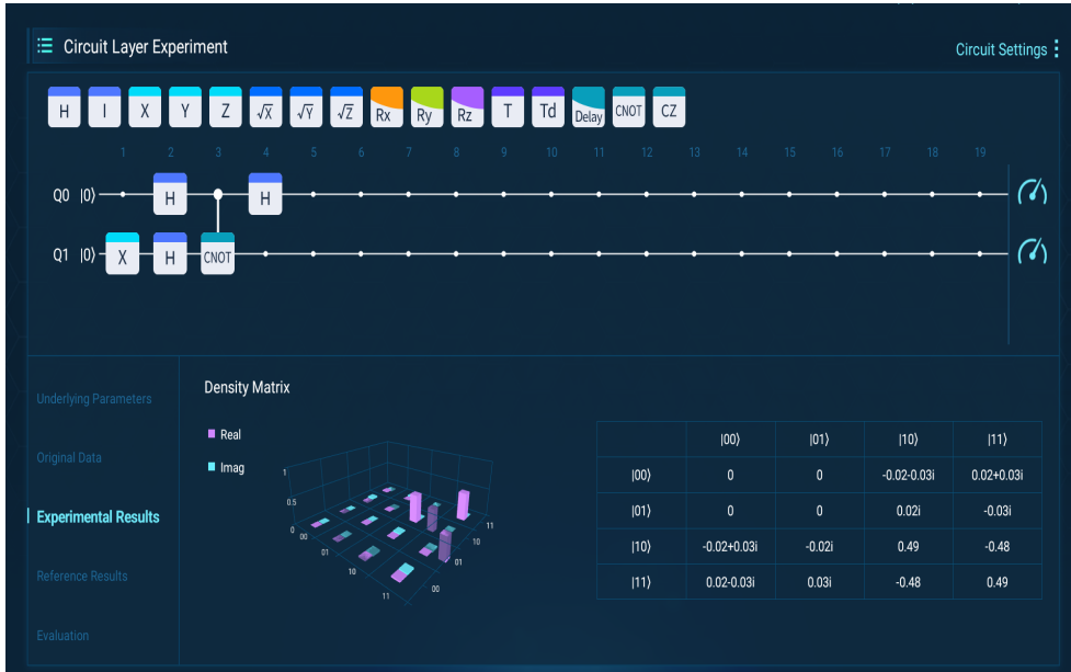
Figure 2. Deutsch algorithm on two qubits.
