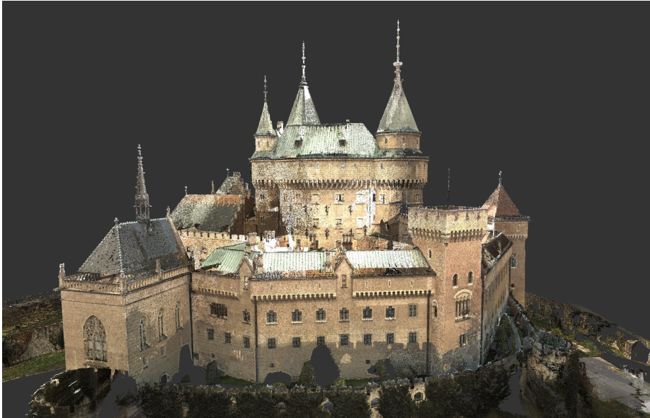
Figure 4. Registered point cloud of a geometrically complex object, after cleaning and segmentation. The figure illustrates the result after removal of noise, moving objects, and irrelevant surroundings.
