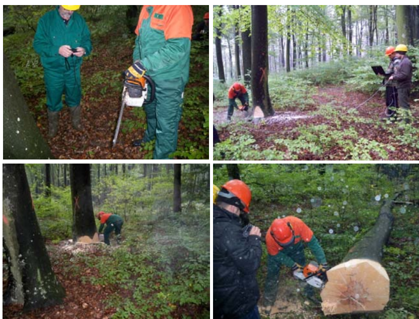
Figure 2: Some activities during handling the chain saw: a) at idling, b) preparing to turn down, c) turning down, d) cross cutting (source: own)
